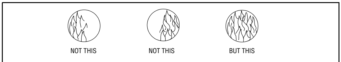
FIGURE 6. FLAME MUST COMPLETELY COVER SIGHT OPENING
